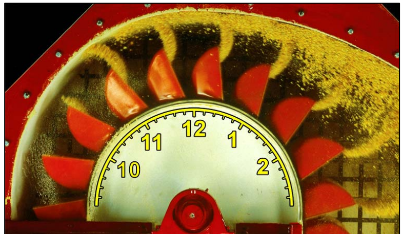
Test Elevator Fitted with Starco Elevator Buckets Showing Initial Discharge at 10 o'clock
